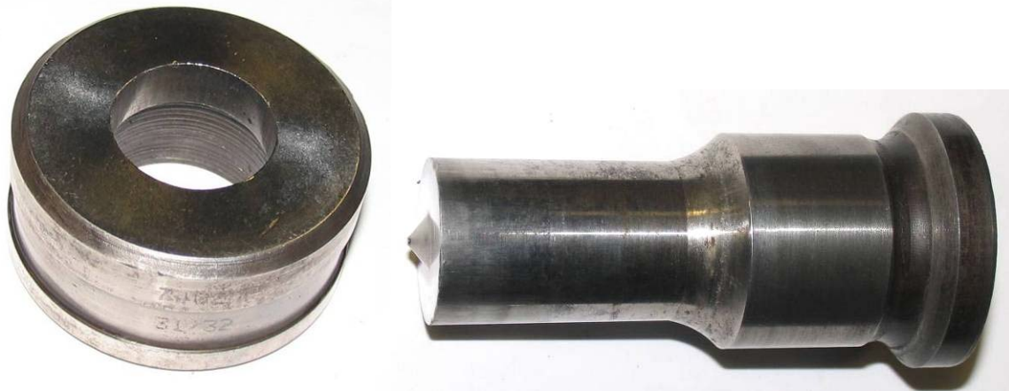
Figure 3.24: 15/16 in. Punch with 31/32 in. Die (At End of Testing)
