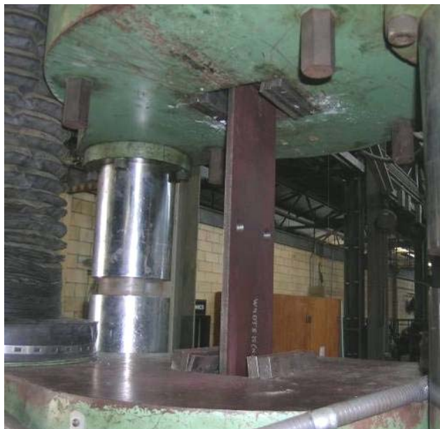
Figure 3.29: Typical Plate Specimen in Universal Testing Machine
