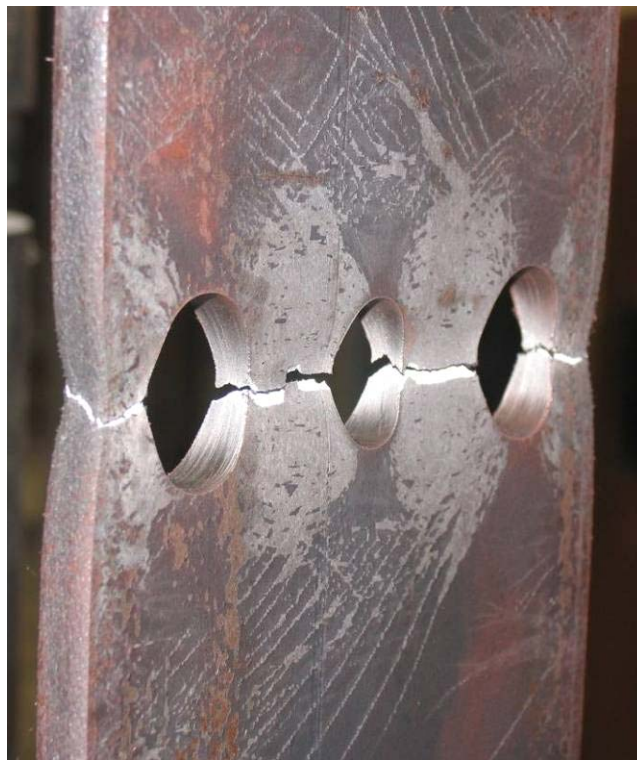
Figure 4.3: Reduced Net Area Plate Specimen Failure—Drilled Holes
