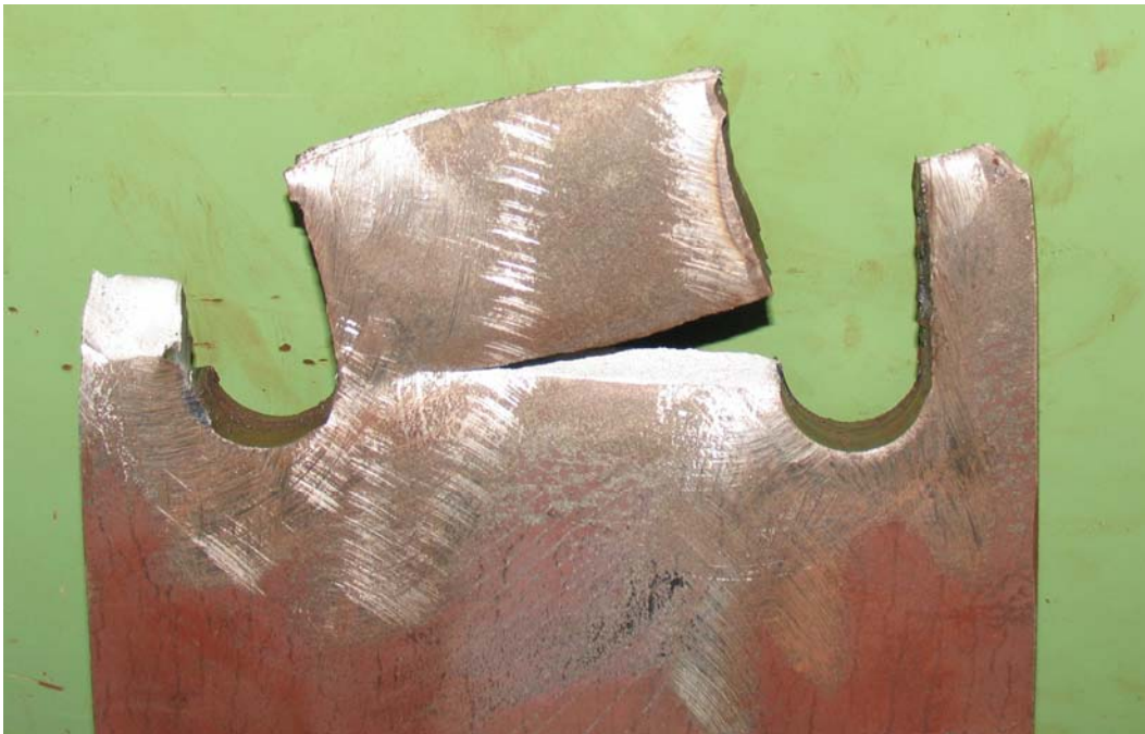
Figure 4.52: Brittle fracture of punched plasma Grade 50 \frac{3}{4} " plate
