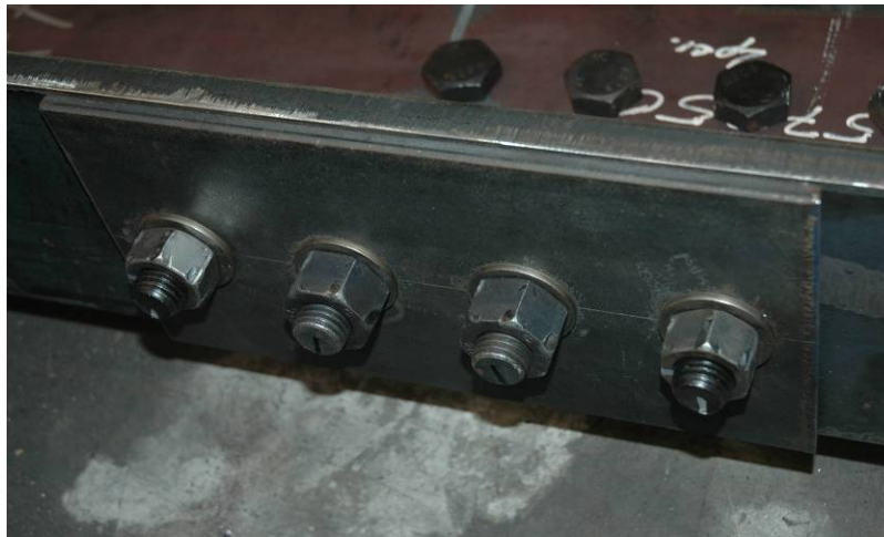
Figure 3.17: Specimen with Bolted Gusset Plate
