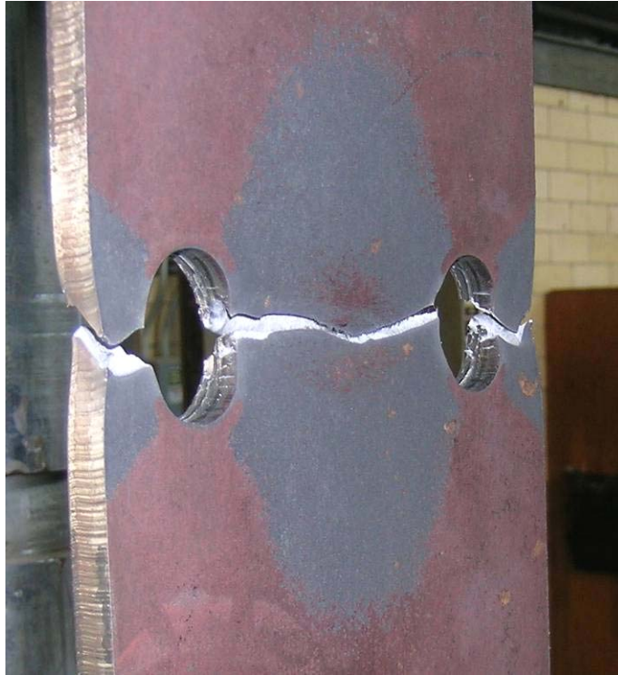
Figure 4.2: Typical Failed Punched Hole Plate Specimen
