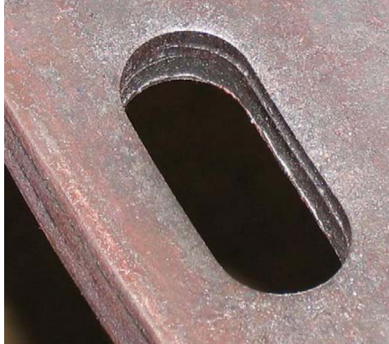
Figure 2.26: Punched slotted hole
