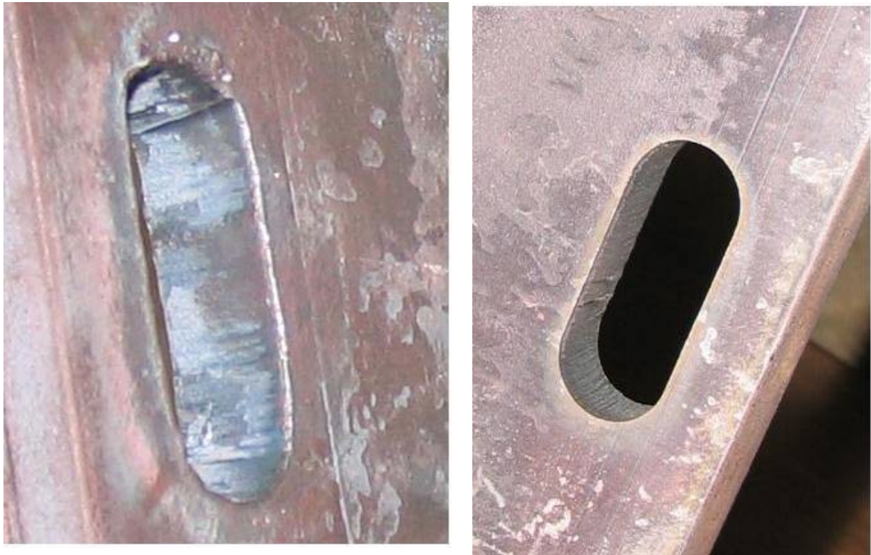
Figure 2.25: Manual oxygen-acetylene(oxy-act)-cut and laser-cut slotted holes
