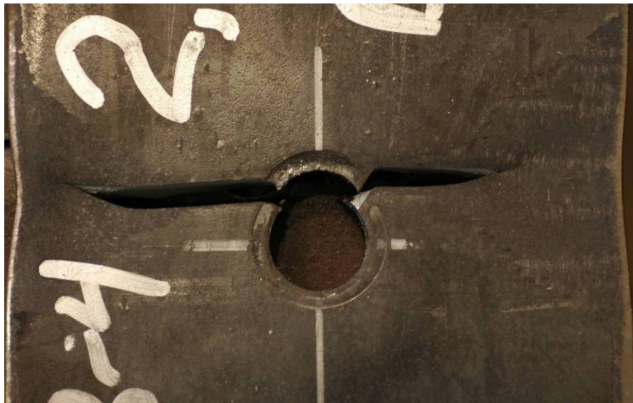
Figure 4.57 Typical Crack Orientation for Thin Plates (<1.0 Inches) with a Gusset Plate (Specimen B-4)
