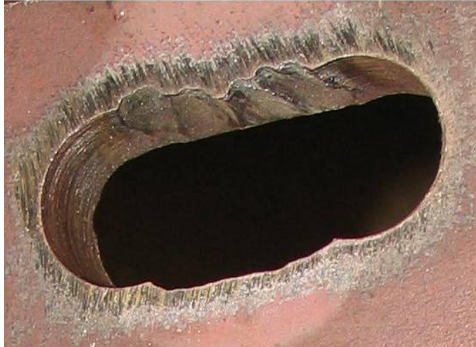
Figure 2.28: Punched holes joined with oxy-act cut
