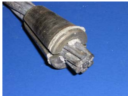
North Duct Strand with Wedges
