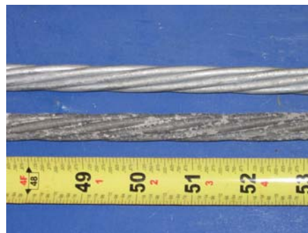
Figure 5.45: Autopsied Galvanized Strand (Bottom) versus New Galvanized Strand (Top)
