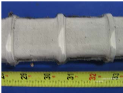
South Duct Grout
