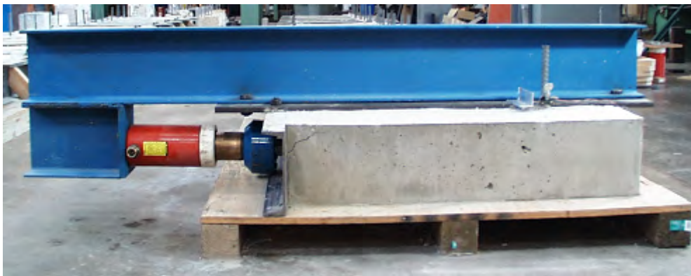
Figure 2.2: Side View of the Push-out Test Setup
