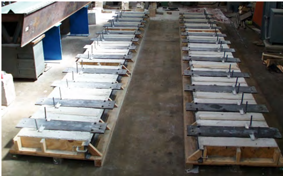
Figure 2.3: View of All Push-out Test Specimens
