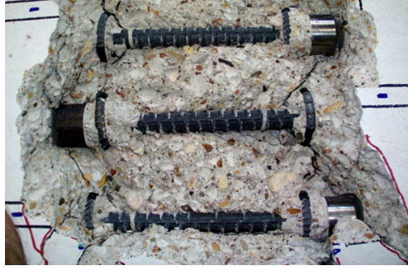
Figure 3-12: Internal cracking with hairpin confinement (specimen LS-08-04.04-12-10(N)-1-H0.6)
