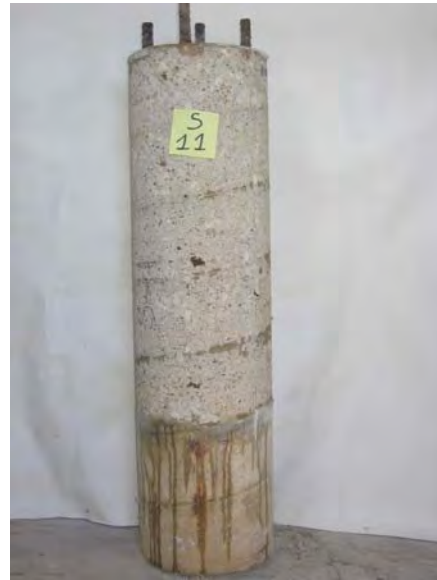
Cylinder S11 after removal of wrap.
