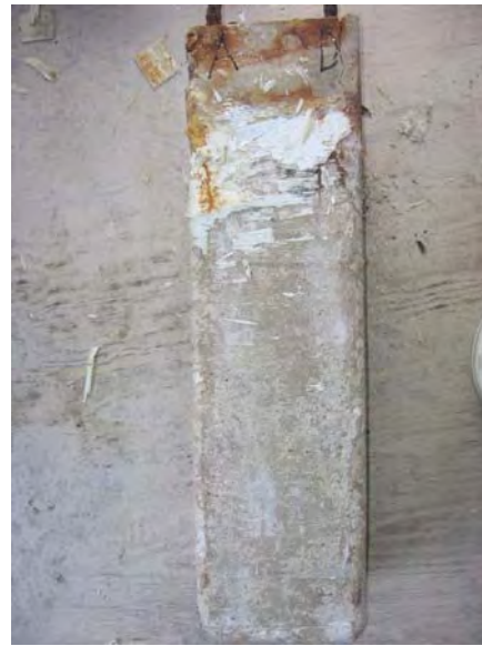
Specimen RNC8 before and after removal of wrap.
