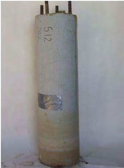
Specimen S12 with wrap intact.
