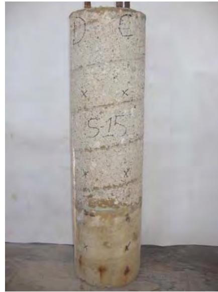
Cylinder S15 after removal of wrap.
