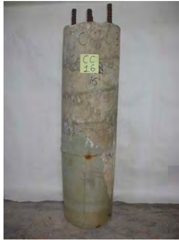
Cylinder CC16 with repair material over bottom region.
