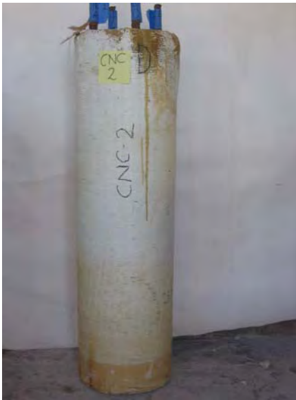
Cylinder CNC2, completely wrapped.
