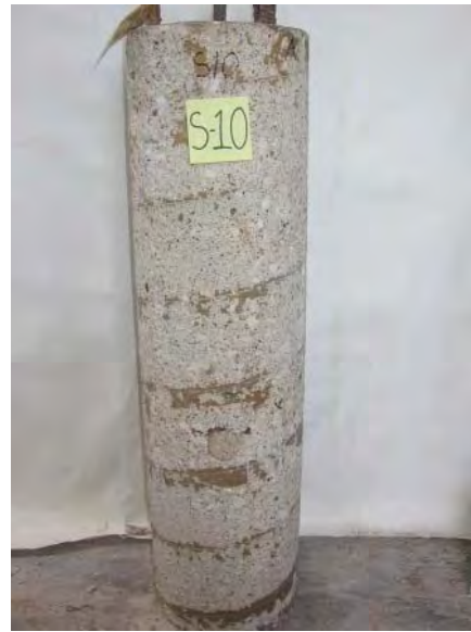
Cylinder S10 after removal of wrap.
