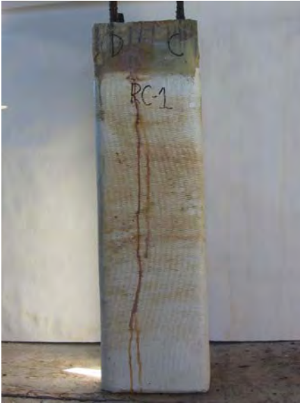
Specimen RC1 wrapped over the top 27 in.
