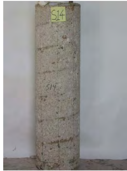
Specimen S14 after removal of wrap.
