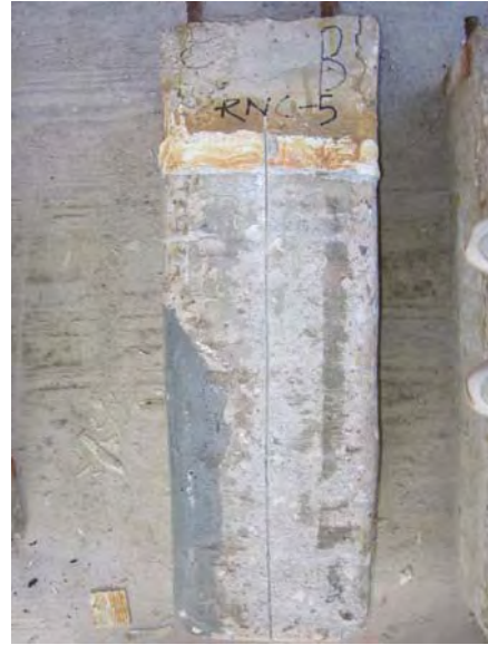
Specimen RNC5 before and after removal of wrap.
