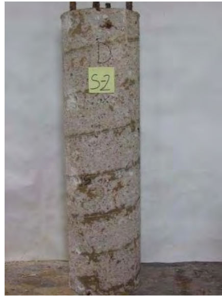
Column S2 after removal of wrap.
