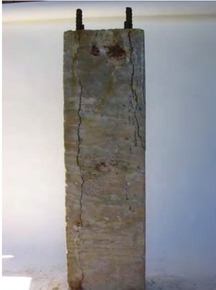
Specimen RC8 with no wrap.
