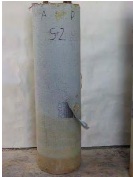
Column S2 Completely wrapped.
