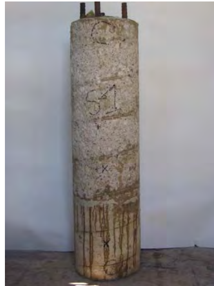
Cylinder S1 after removal of wrap.
