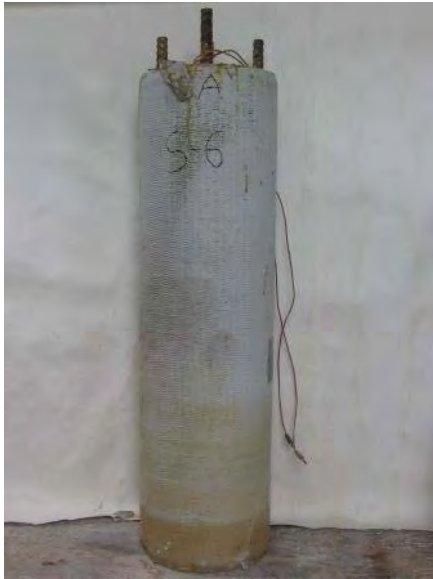
Column S6 completely wrapped.
