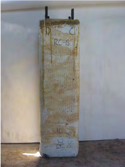
Specimen RC6 wrapped over the top 33 in.
