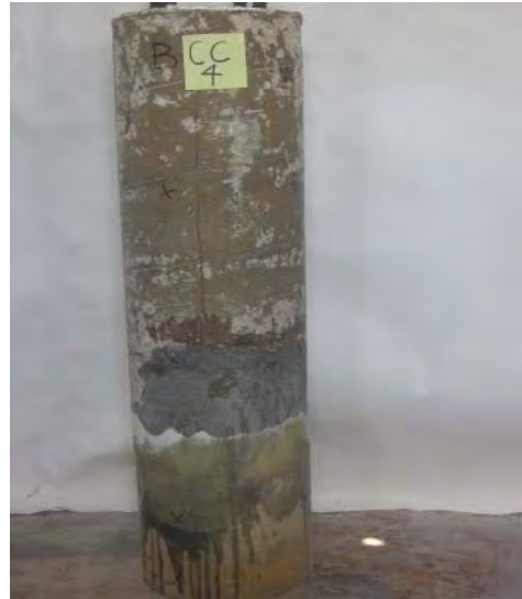
Repair patch over lower portion.
