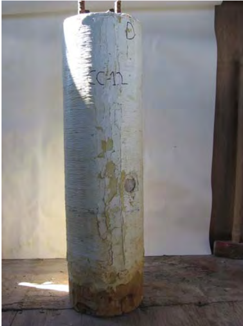
Cylinder CC12 covered with FRP wrap.
