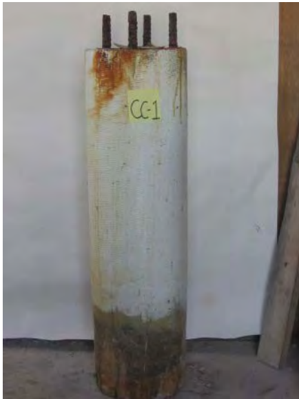
Cylinder CC1 wrapped till 12 in. from bottom.
