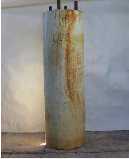
Cylinder CC8 wrapped completely.
