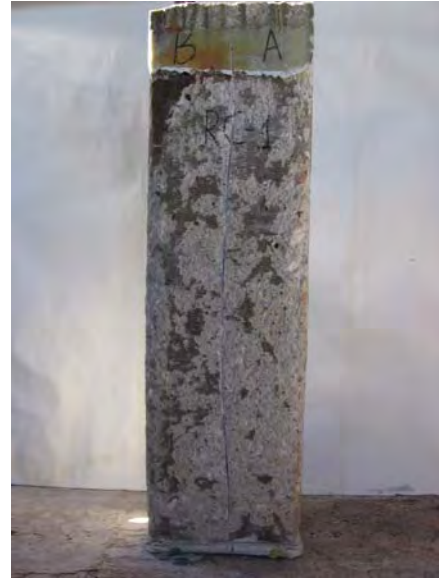
Specimen RC1 with rust stain on rebar B.
