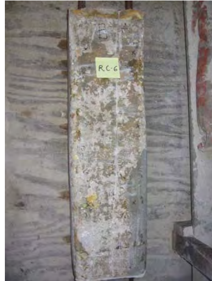
Specimen RC6 after removal of wrap
