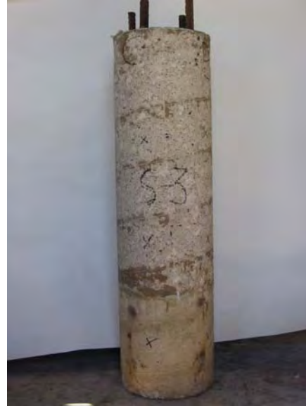
Cylinder S3 after removal of wrap.
