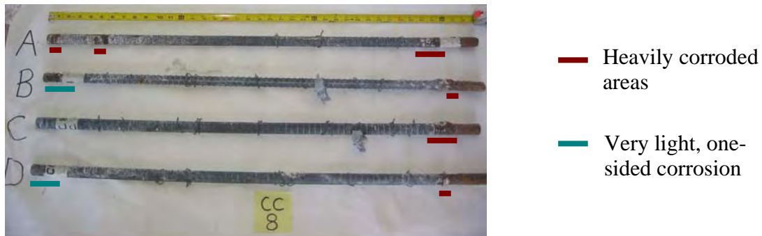
Figure 3.7 Extracted bars from CC8
