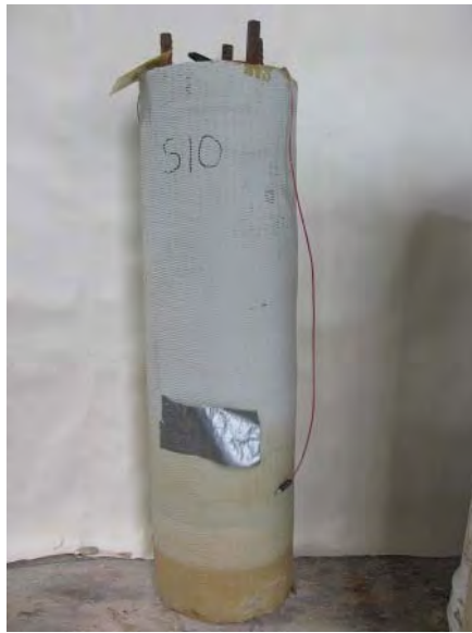
Cylinder S10 completely wrapped.
