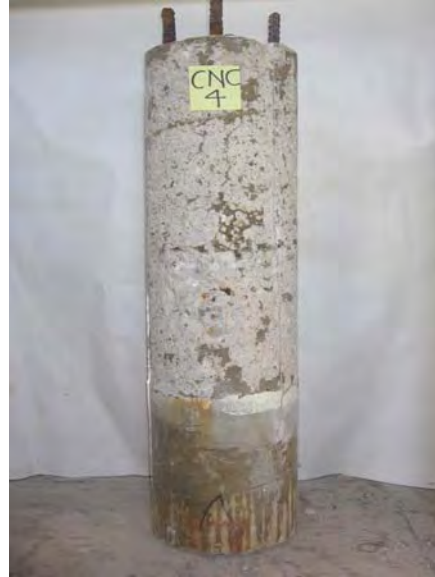
Cylinder CNC4, after removal of wrap.
