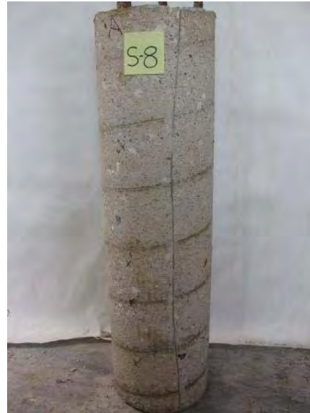
No cracks or rust stains after removal of wrap.
