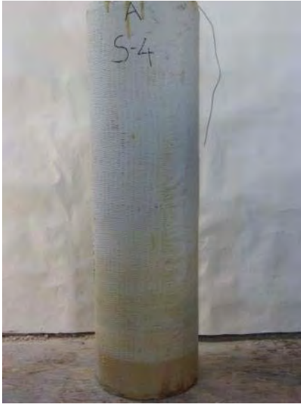
Column S4 Completely wrapped.
