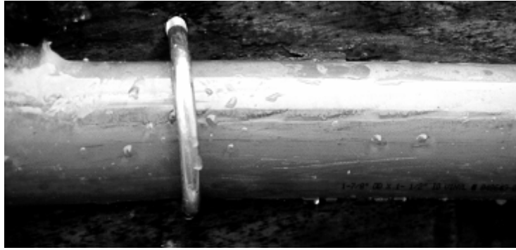
Figure 3.6 Beginning of Void Formation at Intermediate Crest 34
