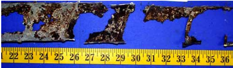
Figure 3.17 Large Galvanized Steel Duct Destruction Due to Corrosion 37,38
