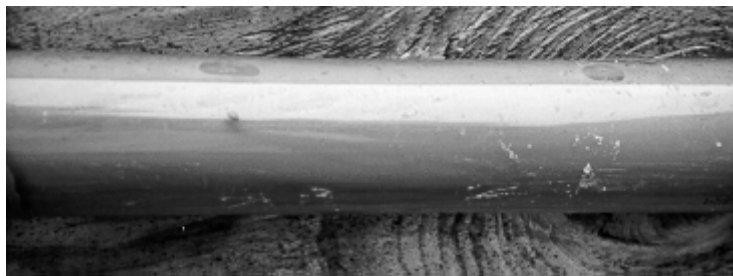
Figure 3.5 TxDOT Grout – Bubbles Traveling Toward Intermediate Crest 34
