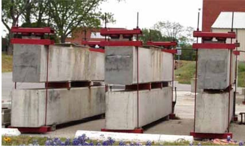
Figure 3.11 Beam Test Setup at North End of Ferguson Laboratory 37
