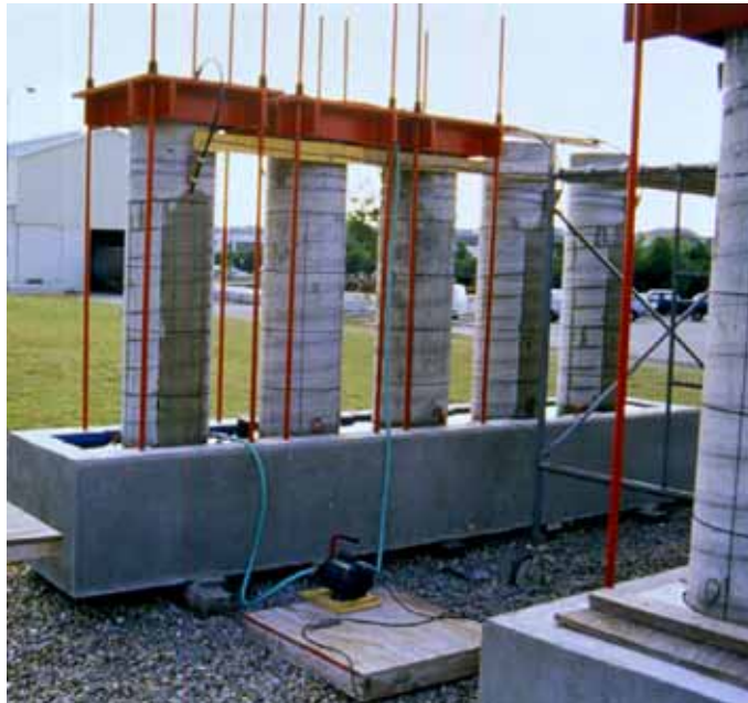
Figure 3.14 Column Test Setup 37
