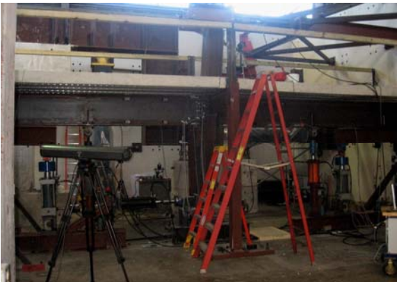
Test setup at 9% inter-story drift
