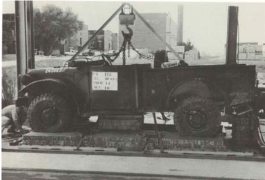
Figure 3: This is a photograph of the truck shown in Figure 2 after the drop. Note how the paper honeycomb cushioning has been crushed in absorbing the shock of the impact.
