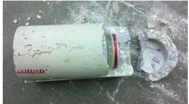
Embedded conductivity sensor in concrete cylinder.
