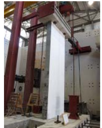
The first quasi-static masonry wall specimen tested.
