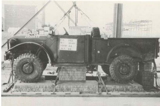
Figure 2: A 3/4-ton truck rigged for a simulated aerial-delivery drop. This vehicle was dropped in free fall from a height of 14 ft.
