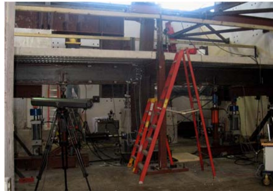
Test Setup at 9% Inter-story Drift
